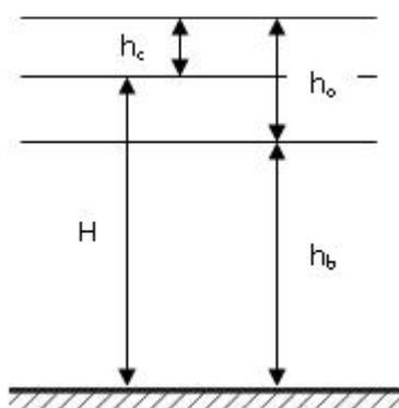
Figure 3 – Measurement of water level in the river by the sensor
