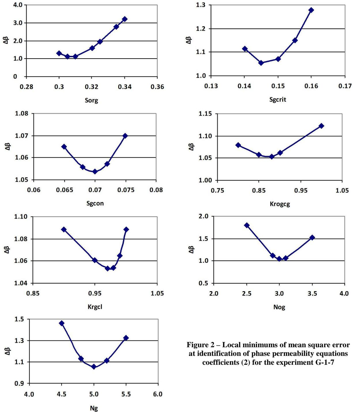
Figure 2 – Local minimums of mean square error at identification of phase permeability equations coefficients (2) for the experiment G-1-7
