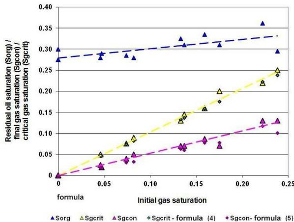
Figure 5 – Interconnection of identified coefficients  $S_{org}$ ,  $S_{gcon}$  and  $S_{gcrit}$  with initial gas saturation
