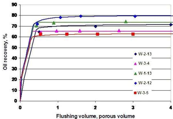
Figure 9 – The results of water-oil displacement simulation for a series of experiments at a sample pressure lower than saturation pressure
