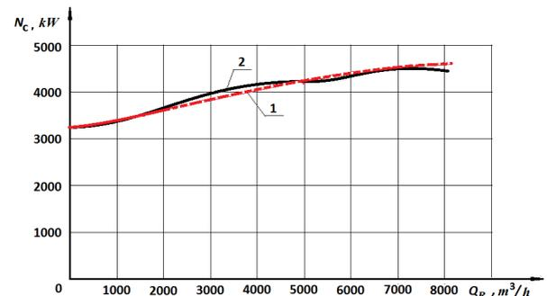
**Figure 8 – The dependence of characteristics of consumed power  $N_c$  on the flow  $Q_R$  of the main pump NM 7000-210 calculated by the presented model (curve 1) and experimentally obtained (curve 2) [17]**
