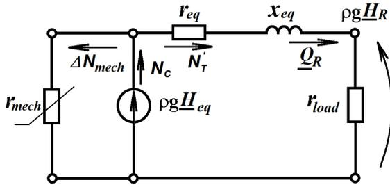
Figure 4 – Equivalent scheme of a CP
