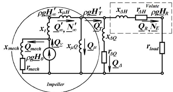
Figure 2 – A complex equivalent circuit of the CP
