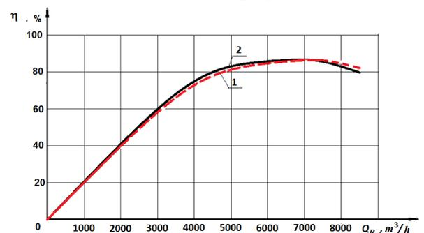
**Figure 9 – The dependence of characteristics of the overall efficiency  $\eta$  on the flow  $Q_R$  of the main pump NM 7000-210 calculated by the presented model (curve 1) and results obtained experimentally (curve 2) [17]**
