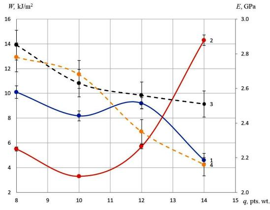
(1)  $T = 393 \pm 2 K$  and (2)  $T = 413 \pm 2 K$  – the modulus of elasticity during the flexion (E) of the polymer matrix, hardened at a temperature: (3)  $T = 393 \pm 2 K$  and (4)  $T = 413 \pm 2 K$
