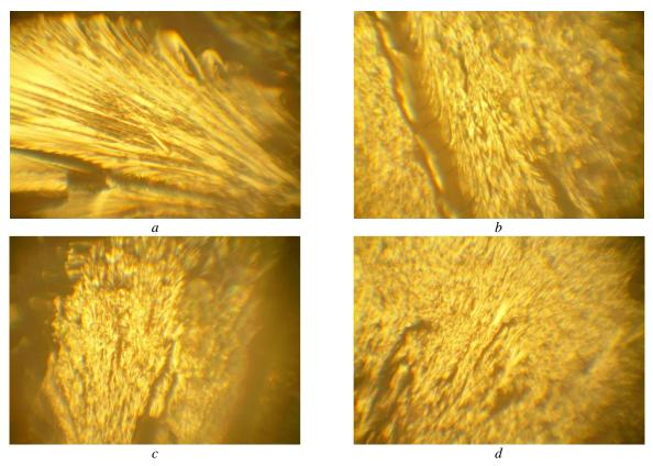
a) 8 weight parts, b) 10 weight parts, c) 12 weight parts, d) 14 weight parts Figure 4 – Fracture pattern of the polymer matrix hardened at a temperature T = 413 ± 2 K with usage of PEPA hardener
