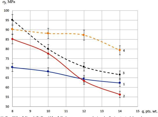
(1)  $T = 393 \pm 2 K$  and (2)  $T = 413 \pm 2 K$ ; fracture stresses during the flexion ( $\sigma_{fl}$ ) of the polymer matrix, hardened at a temperature: (3)  $T = 393 \pm 2 K$  and (4)  $T = 413 \pm 2 K$
