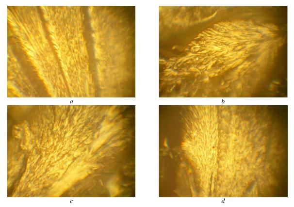
a) 8 weight parts, b) 10 weight parts, c) 12 weight parts, d) 14 weight parts Figure 5 – Fracture pattern of the polymer matrix hardened at a temperature T = 393 ± 2 K with usage of TETA hardener
