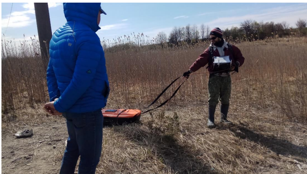
Fig. 5. The geo-radar sensing in Starunja (photo by I. I. Kovbaniuk)
